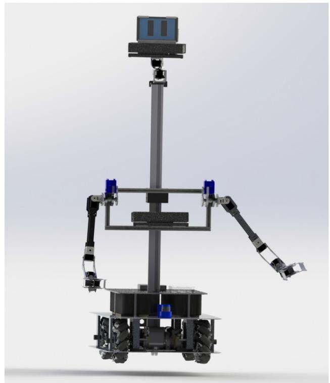
Figure 4: The robot can move the torso until the arms reach an object on the floor.
