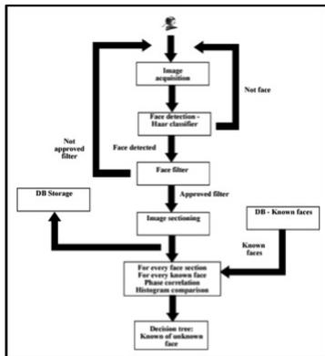
Figure 6: Face Recognition Algorithm.
