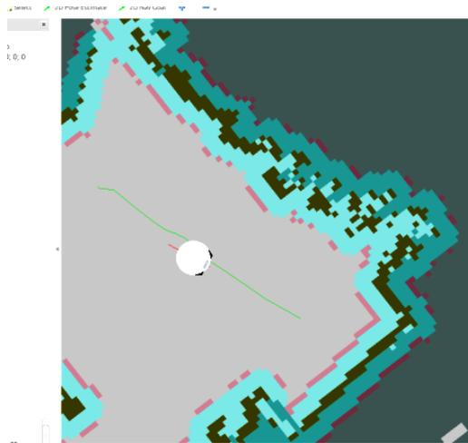
Figure 4 Turtlebot path planning after the use of SLAM algorithm
